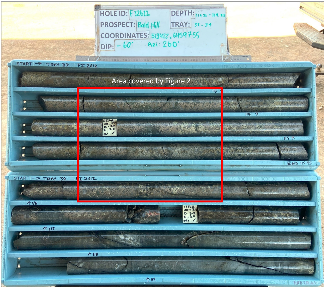
Figure 1: FI2612 diamond (NQ) drill core from 112.32 to 119.45 metres showing semi-massive sulphides from 112.32 metres to 117.40 metres. The location of Figure 2 is shown by the red square.
