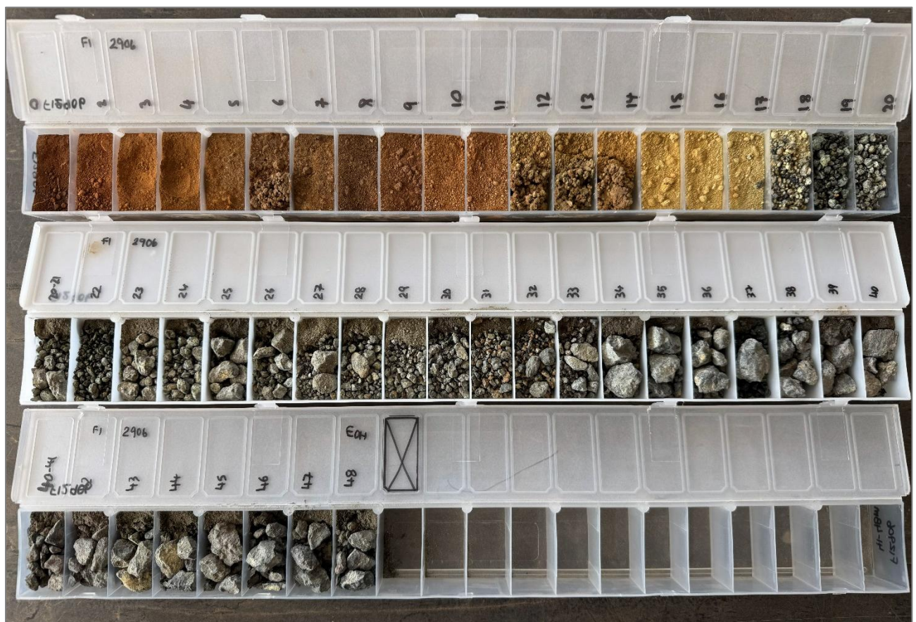
Figure 6: Photograph of chip trays from FI2906 that was drilled at the Murga Exploration Target during the recent program. Each interval represents 1 metre of drilling. The hole shows laterite and saprolite clays developed over moderately to weakly weathered pyroxenite rocks (saprock) from 18 metres downhole. Also refer to Table 3 for individual scandium assay values.
