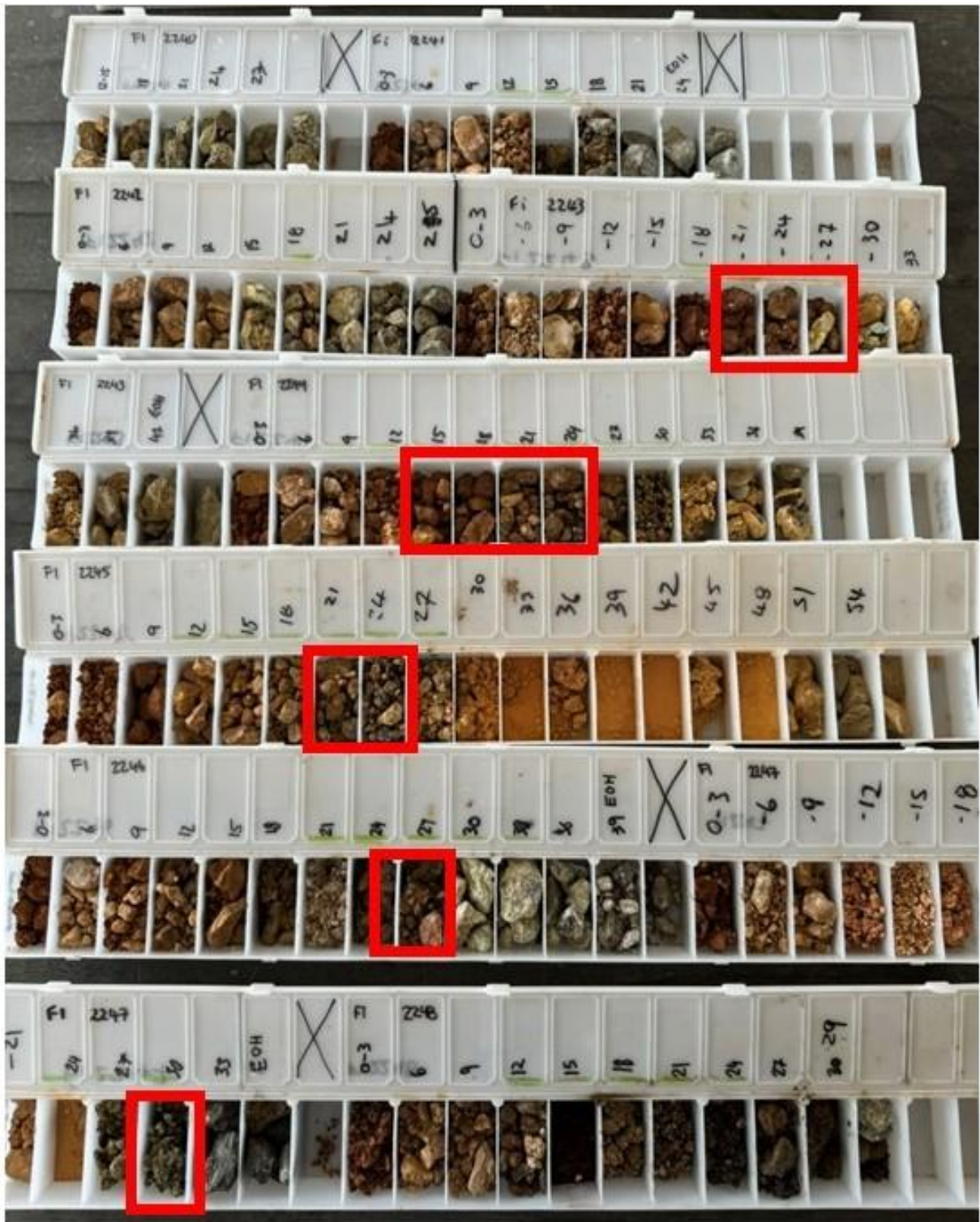
Figure 6: Currajong Prospect chip trays showing anomalous scandium (+100ppm Sc) intervals. Note each interval represents 3 metres downhole.
