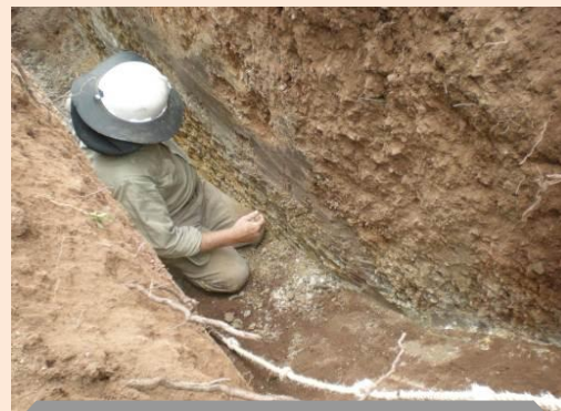
Bedrock breccia zone in a 13m trench (31) located on Auger traverse section FiAug 822-824 with good Au assay
