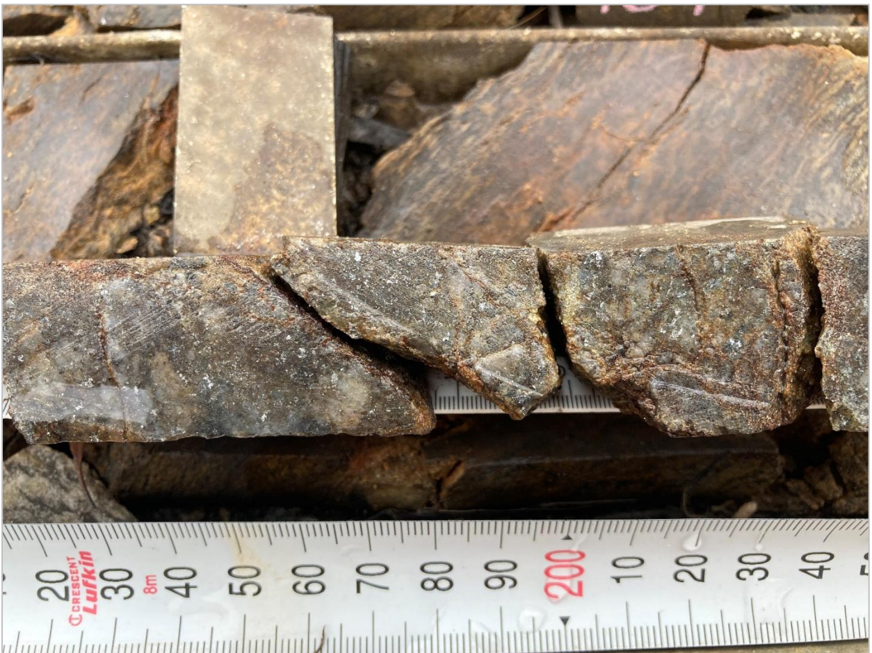
Figure 1: Close up photographs of NQ diamond quarter core for 189.40 metres in NPD1 – D1 showing strongly disseminated arsenopyrite (silver flecks) within a sheared and brecciated quartz - chlorite rock.
