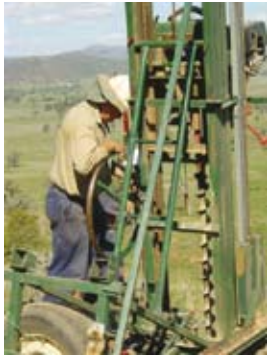
Auger Drilling Tom & Jerry Mountain area
