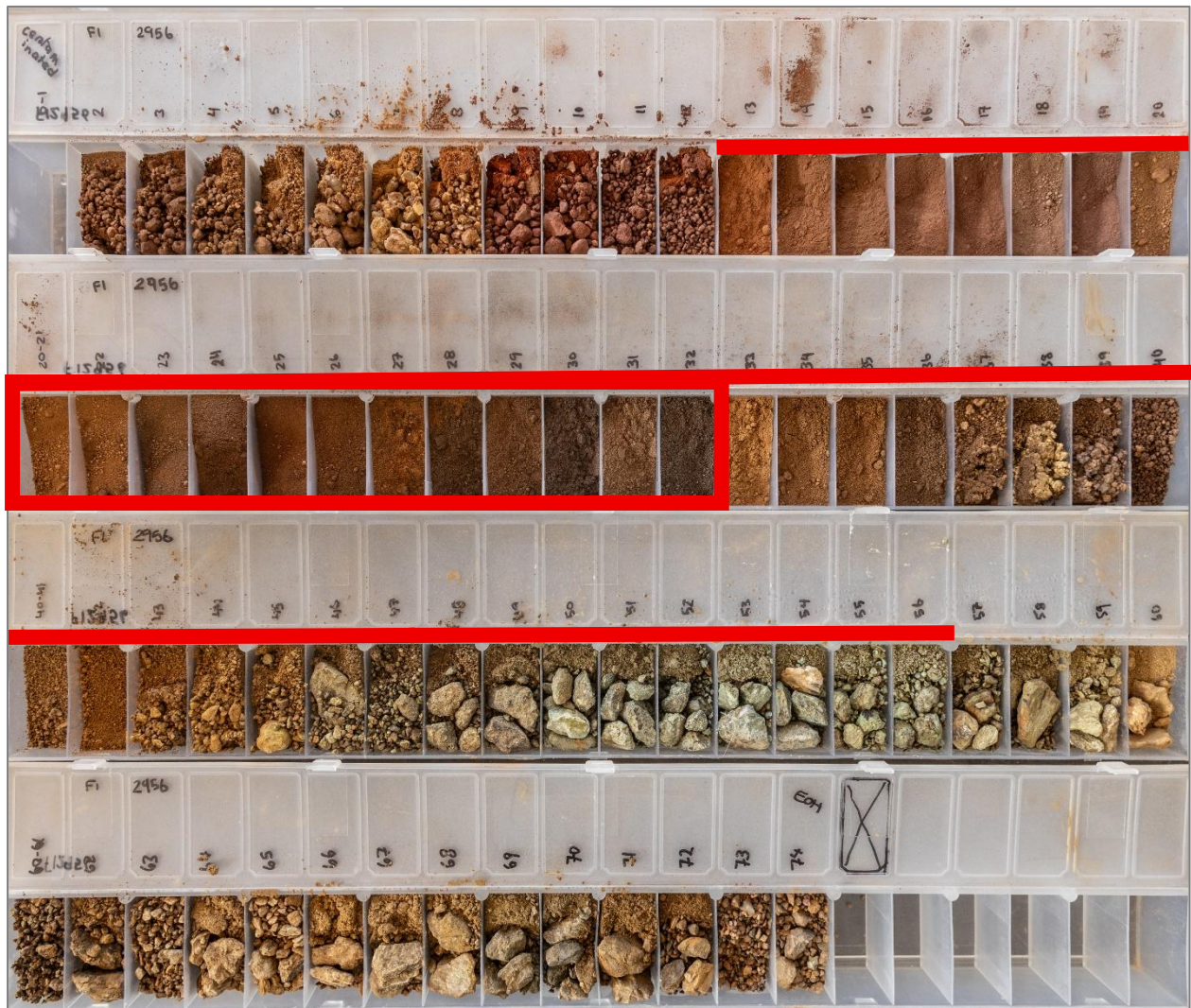
Figure 5a: Photograph of chip trays from FI2956 that was drilled at the Malamute Scandium Prospect. Each interval represents 1 metre of drilling. Red highlighted portion denotes scandium intercept of - 44m @ 175ppm Sc (268ppm Sc Oxide) from 12 metres in FI2956 including 12m @ 281ppm Sc (431ppm Sc Oxide) ,
