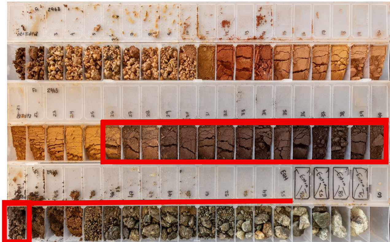
Figure 5b: Photograph of chip trays from FI2963 that was drilled at the Malamute Scandium Prospect. Each interval represents 1 metre of drilling. Red highlighted portion denotes scandium intercept of -30m @ 247ppm Sc (378ppm Sc Oxide) from 25 metres in FI2963 including 16m @ 352ppm Sc (540ppm Sc Oxide)
