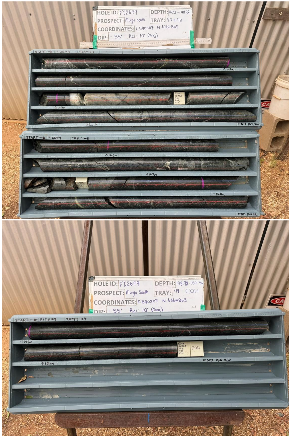
Figure 6b: FI2679 – photos of diamond drill core 142.2 to 150.5 metres EOH. (lower Sc enriched pyroxenite zone)
