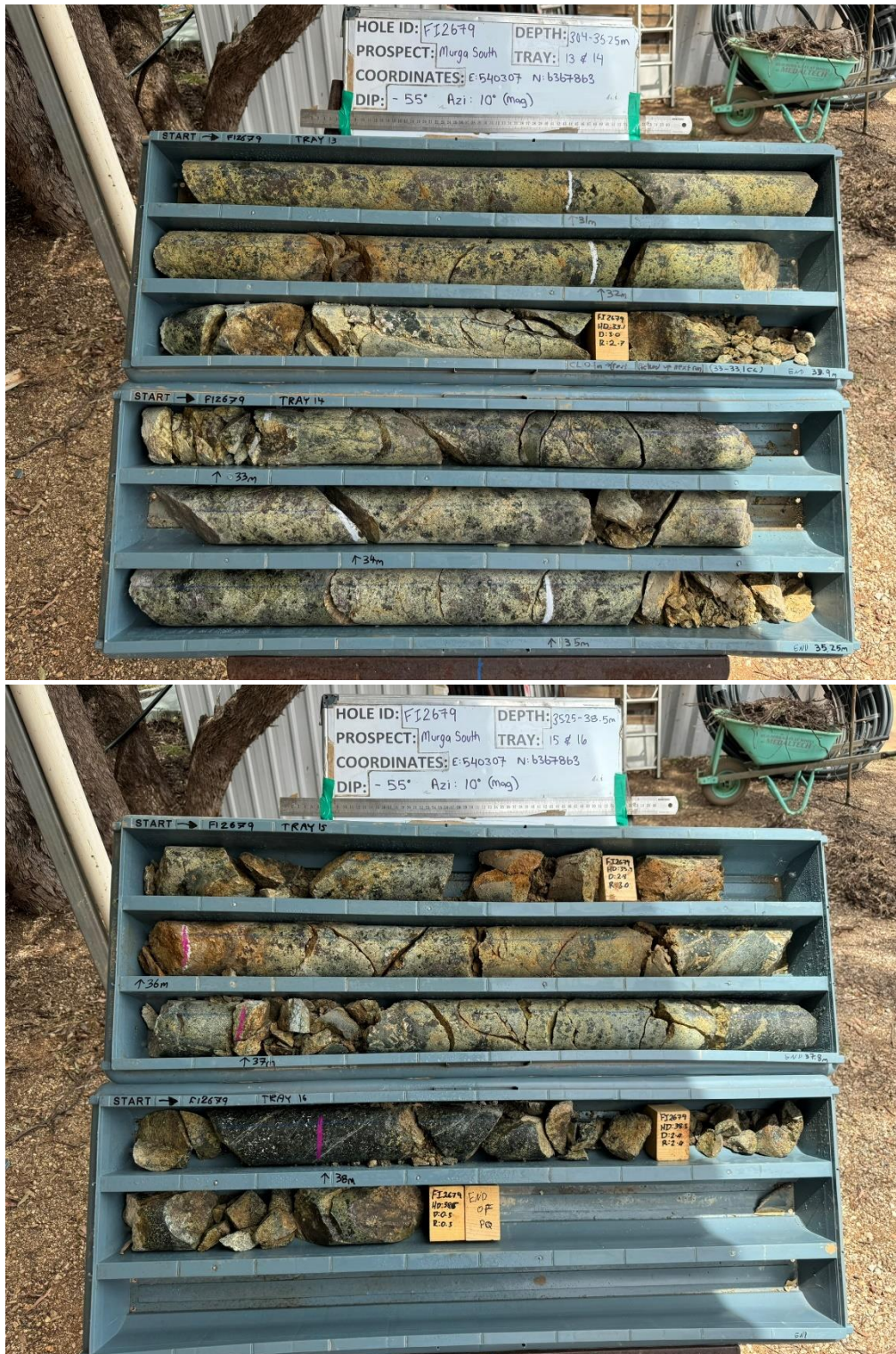
Figure 5d: FI2679 – photos of diamond drill core 30.4 to 38.5 metres (lower saprolite / saprock)
