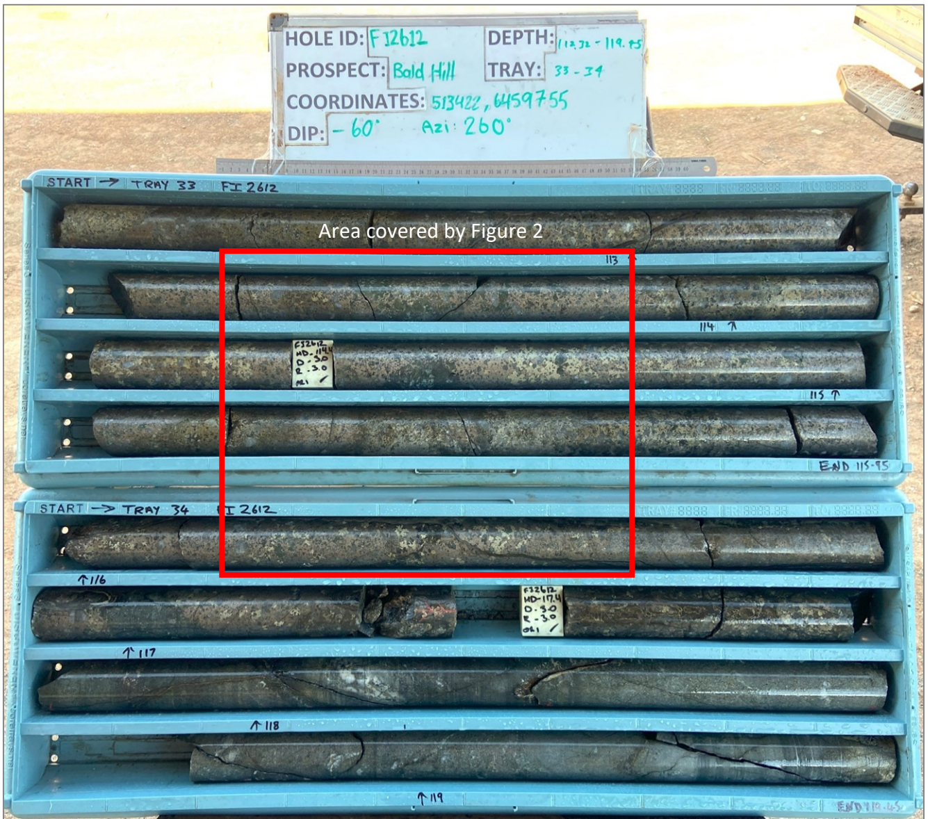
Figure 1: FI2612 diamond (NQ) drill core from 112.32 to 119.45 metres showing semi-massive sulphides from 112.32 metres to 117.40 metres. The location of Figure 2 is shown by the red square.
