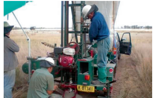
Auger drilling into bedrock – Coherent Au zones
