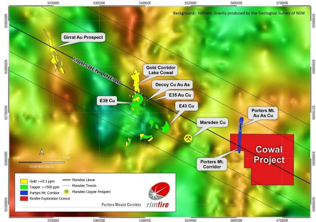
Porters Mount corridor is intersected by Marsden Linear and on a N-S structure that is parallel to Cowal N-S structure.
