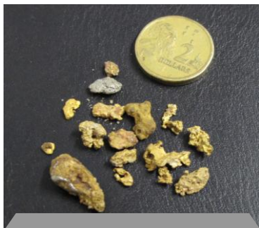
9g “oversize” Pt & Au from Platina Lead Clay Dump, Trial 17t sample
