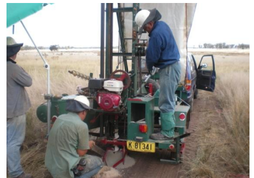
Auger drilling into bedrock – Coherent Au zones
