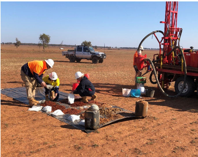
Aircore Drilling at Northern Area. Drilling technique requires no disturbance of topsoil and excess sample is put back in hole on completion of sampling
