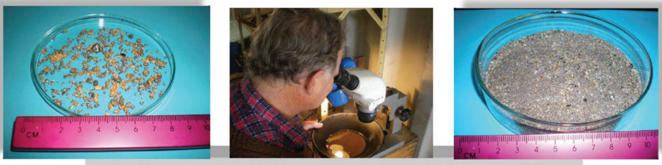
Examining clean precious metal concentrates where coarse (left) and fine (right) Pt and Au have been recovered, with selected material being refined (approx. 400g) or undergoing further petrological testing.
