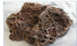
Figure 1: Rock Chip sample FIR1681 displaying lattice texture indicative of boiling.
