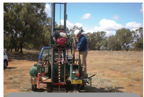
Delineating areas with Auger Drilling
